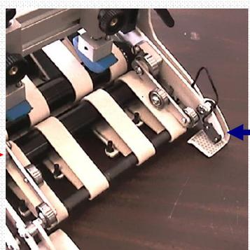
*Our Patented paper guide extensions guide the document right into the gripper, eliminating extra components and touchy photo eye adjustments!*
